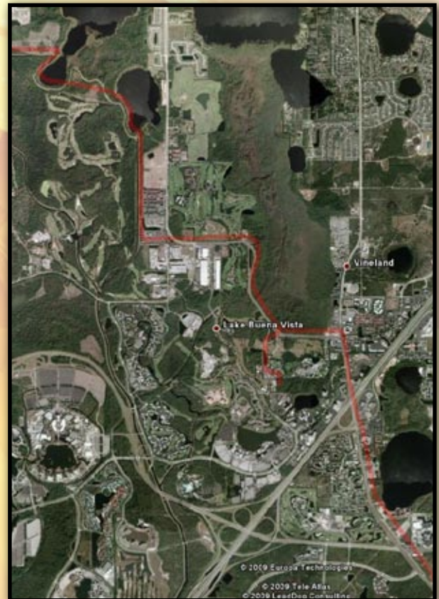
Rextag's Pipeline GIS Data (Red Line) at 101' - 500'. 18% Acceptable Accuracy
