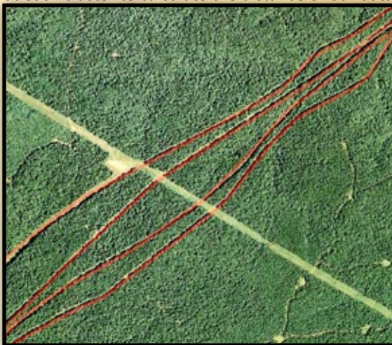
Rextag's Pipeline GIS Sample (Red Lines) Perfectly Overlaid on Aerial Photography's Pipeline ROW "Scars" (38% at 0' to 10' Perfect Accuracy)
